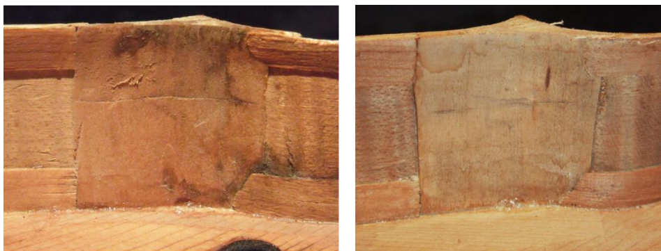
Figure 8. Corner blocks have a knife cut score as the maker's habit in trimming the blocks with the presence of internal mould.
