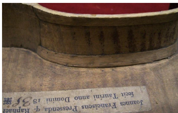
Figure 6. In interior, the surface of a C bout rib shows a stained feature of liquid varnish penetrated from the external surface as a result of ideosyncratic recipe of varnish coating.
